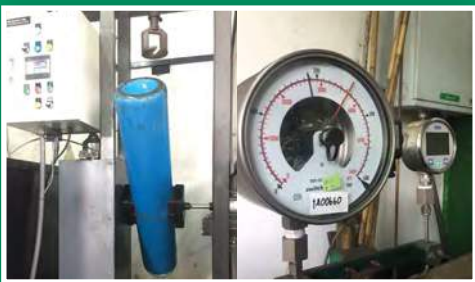
Cylinder hydrostatic test every 5 years for safe operation of cylinder
